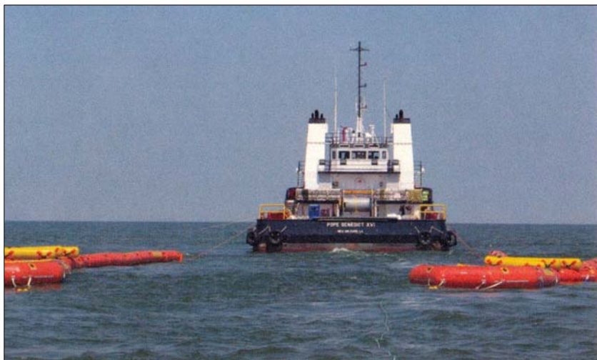
A Current Buster is towed behind the Pope Benedict XVI in skimming operations. The OSV, owned by Adbon Callais Offshore LLC, is under contract with BP for recovery operations.
